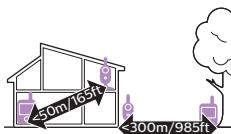
The operating range is up to 50 meters / 165 feet indoors and 300 meters / 985 feet outdoors. The operating range of the baby monitor varies depending on the surroundings and factors that cause interference. Wet and moist materials cause so much interference that the range loss is up to 100%.
