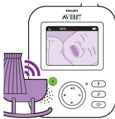
When sound is picked up by the baby unit, the display and sound of the parent unit switch on immediately. The sounds are transmitted to the parent unit.
